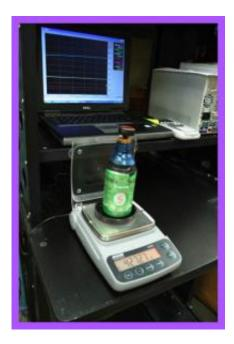
A test subject being weighed to measure the amount of condensation. The cap prevents air from moving through the opening on top.
