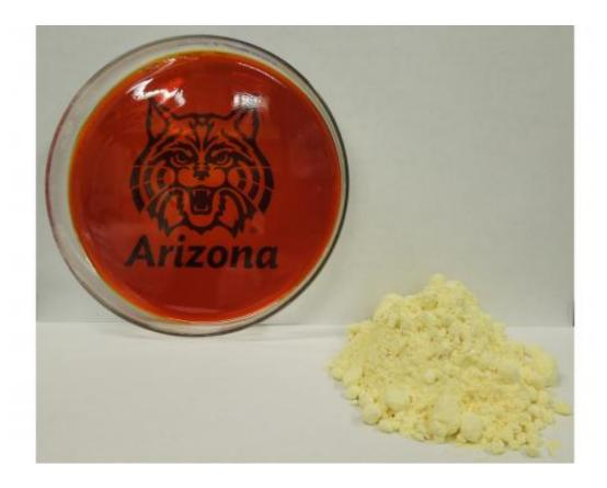
A University of Arizona-led research team has discovered a simple process for making a new lightweight plastic from the inexpensive and abundant element sulfur. The petri dish on the left contains the plastic. The yellow powder on the right is sulfur. The team has already made a lithium-sulfur battery -- the type of next- generation battery that is lighter and cheaper than those currently used in electric and hybrid cars. Credit: Jared Griebel/ Pyun lab, University of Arizona
