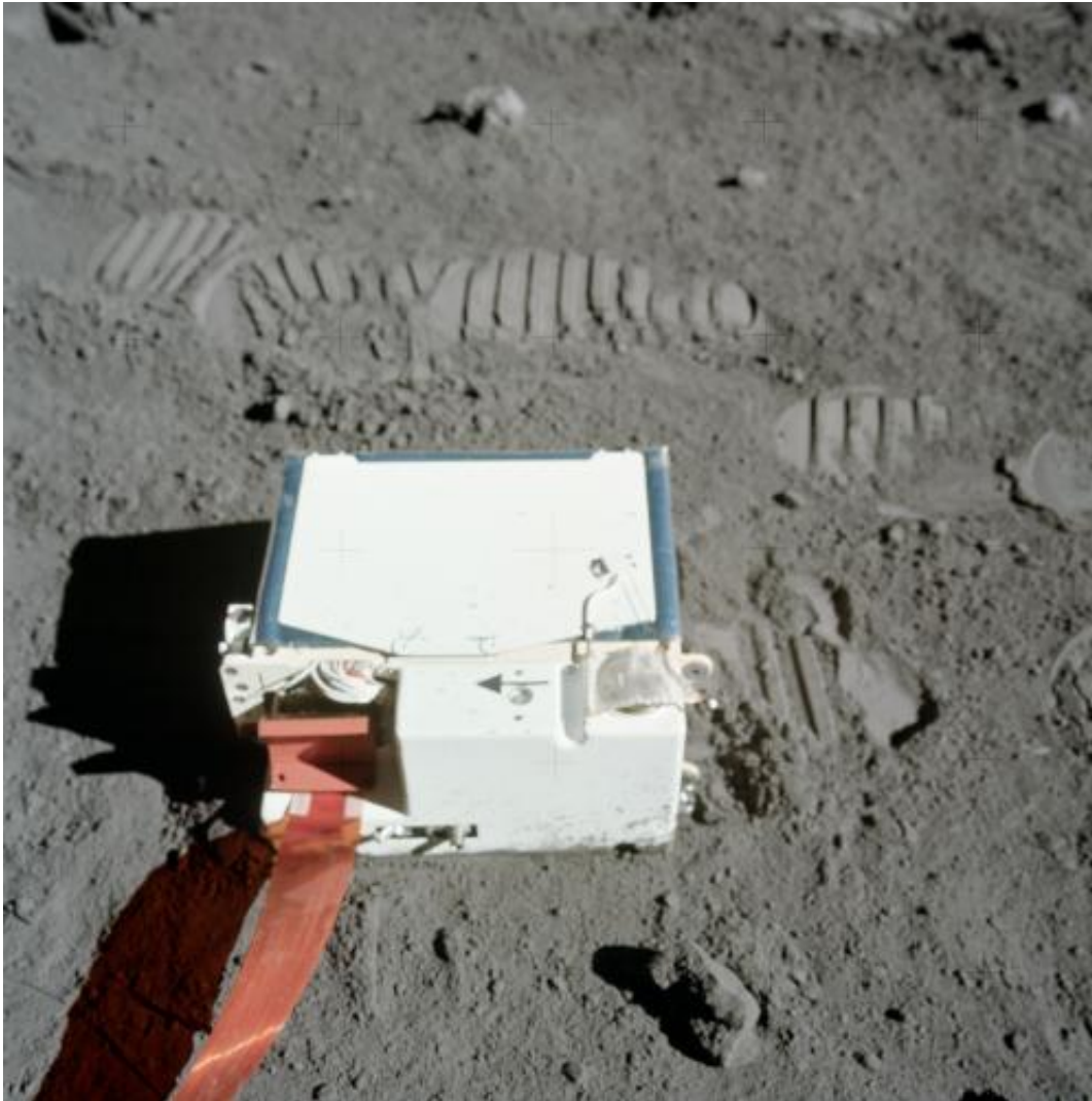
The Lunar Atmospheric Composition Experiment (LACE) deployment during the Apollo 17 mission. Credit: NASA
