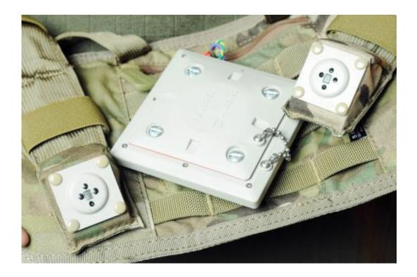
Components of the Integrated Blast Effect Sensor Suite (IBESS) are shown. The system measures the physical environment of an explosion and collects data that can be used to correlate what the soldier experienced with long-term medical outcomes. Credit: Gary Meek
