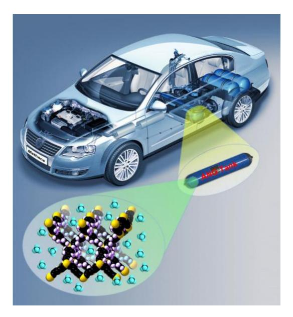
An illustration of a prototype 6-liter adsorbed natural gas (ANG) fuel tank that relies on innovative advanced porous materials and Texas A&M's proven expertise in metal-organic frameworks (MOF) and porous-polymer networks (PPN) to deliver low-pressure, high-density natural gas storage in vehicles.
