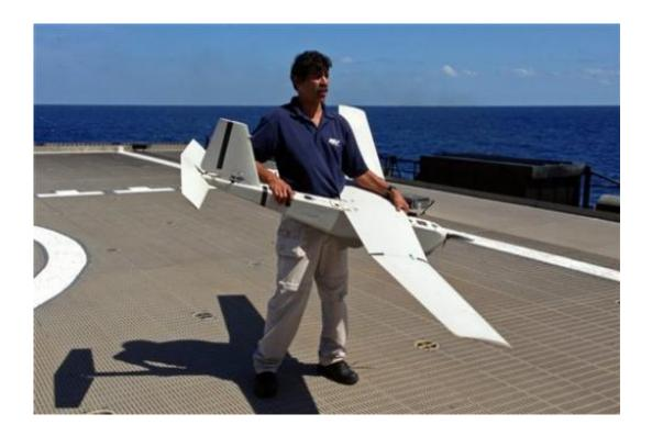
Stuart Orozco, flight operator with Aeronvironment Inc., prepares lo launch a UAS (unmanned aircraft system) named Puma from the deck of the U.S. Navy high speed vessel Swift near Key West, Florida, Friday, April 26, 2013. The U.S. Navy on Friday began testing two new aerial tools, borrowed from the battlefields of Afghanistan and Iraq, that officials say will make it easier to detect, track and videotape drug smugglers in action. (AP Photo/Ben Fox)
