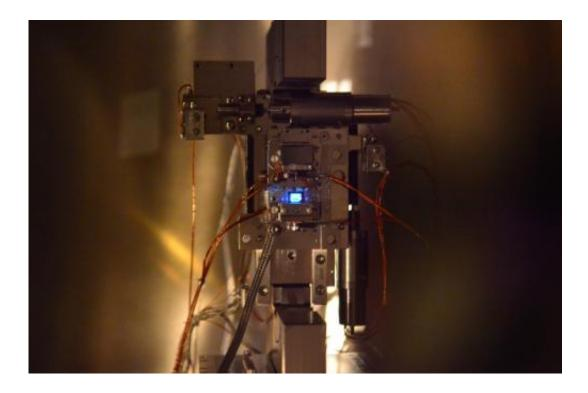
A superthin diamond glows blue during a beam-sharing experiment at SLAC's Linac Coherent Light Source X-ray laser. Credit: SLAC
