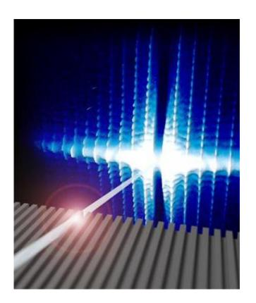
This rendering shows the high-intensity x-ray beam striking and then traveling through the gray sample material. In this new technique, the x-ray scattering—the blue and white ripples—is considerably less distorted than in other methods, producing superior images with less complex analysis.
