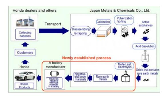
Honda's process for recycling nickel-metal hydride batteries.
