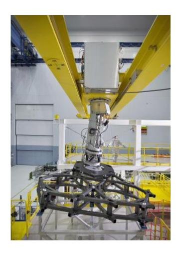
A surrogate mirror segment which is the same hexagonal shape and same mass or weight as one of the primary flight mirrors, is being carefully attached to the a test structure called a "backplane" that will hold 18 of those mirrors on the Webb telescope. Credit: NASA/Chris Gunn
