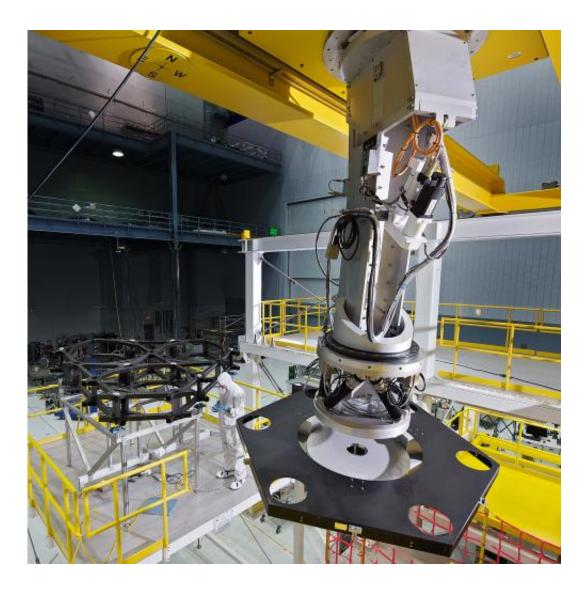
The robot arm moves the surrogate mirror segment (black hexagonal shape) to the test backplane for placement. Credit: NASA/Chris Gunn
