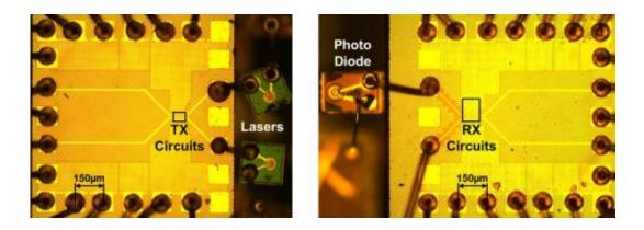
This shows optical link test chips, including transmitter circuits, laser diodes, photo diode, and receiver circuits. Credit: Image courtesy IBM
