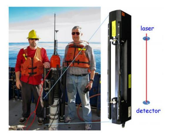
Todd Wood (left) and Jim Bishop with a Carbon Explorer. Particles in the water flow through the PIC sensor's open channel as the Explorer drifts with the current. Polarizing filters, one near the source of the laser beam and the other over the detector, together block all light except what calcium carbonate refracts. Calcium carbonate twists transmitted light, allowing it to pass through the second filter to be recorded on the detector. Credit: Alex Derr
