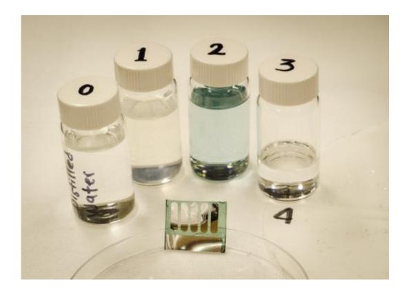
Georgia Tech has created a recyclable solar cell on nanocellulose substrates made from trees. Also pictured are vials that contain the different parts of the cell after it was dissolved in water and the organic solvent. Credit: Canek Fuentes-Hernandez, Georgia Tech
