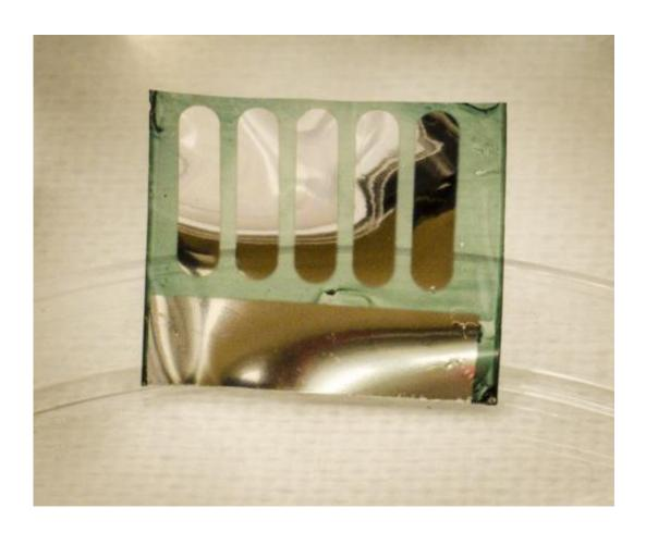
This is a photograph of a solar cell fabricated at Georgia Tech on nanocellulose substrates derived from trees. Credit: Canek Fuentes-Hernandez, Georigia Tech
