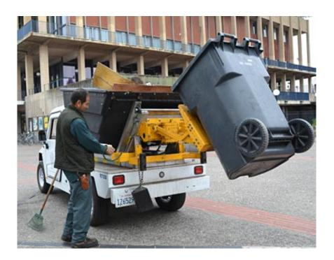
Gardener Juan Casanova transfers trash to a one-of-a-kind vehicle equipped with a tipping mechanism and hopper.
