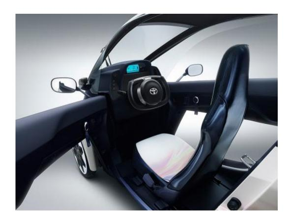
The i-Road leans itself over like a scooter in navigating, when needed, in a self-leaning system that can automatically balance the vehicle. The system allows the two front wheels to move independently of each other. With the aid of computer-controlled technology, the system can figure
