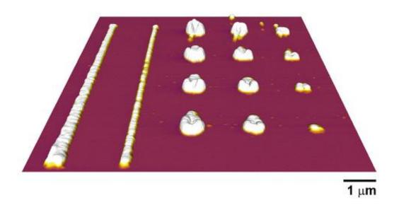
The chemical properties of these polymer nanostructures were measured using atomic force microscope infrared spectroscopy (AFM-IR). Credit: University of Illinois at Urbana-Champaign
