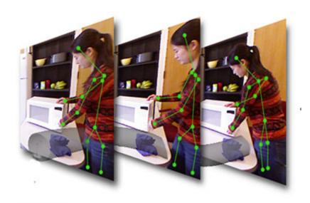
For easy calculation a robot simplifies the image of a human to a skeleton of dots and lines. The volume around the hands is examined to see what object the human is using. Credit: Saxena Lab
