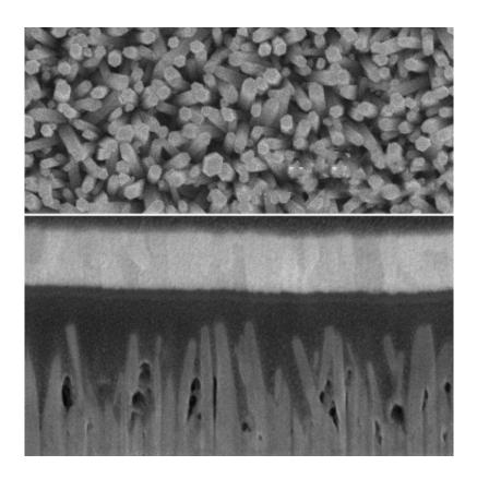
Scanning Electron Microscope images show an array of zinc-oxide nanowires (top) and a cross-section of a photovoltaic cell made from the nano wires, interspersed with quantum dots made of lead sulfide (dark areas). A layer of gold at the top (light band) and a layer of indium-tin-oxide at the bottom (lighter area) form the two electrodes of the solar cell. Credit: Jean, et al. *Advanced Materials*
