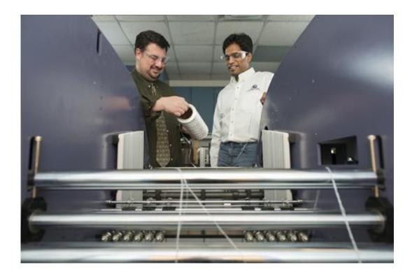
Mark Mirotznik (left) and Shridhar Yarlagadda work at the computerized loom in the Composites Manufacturing Science Laboratory at UD, which enables the researchers to make a broad array of custom composite fabrics for multifunctional structures.
