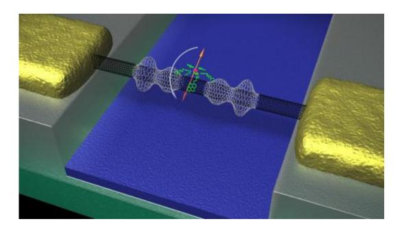
The spin of a molecule (orange) changes and deforms the nanotube (black) mounted between two electrodes (gold). Credit: C. Grupe/KIT
