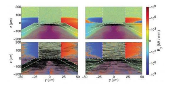
These images from their simulations highlight the trajectories of randomlyselected electrons for a thin cone (left) and thick cone (right), each attached to a copper wire. Background colors show the strength of the electric fields pointing away from the cone and wire. For thin cones, the electric fields act to guide energetic electrons forward into the wire while for thick cones -- a more realistic case -- these fields are too distant to be effective. Credit: Ohio State
