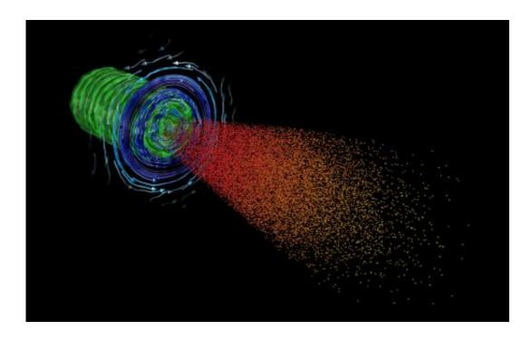
OSIRIS simulation on Sequoia of the interaction of a fast-ignition-scale laser with a dense DT plasma. The laser field is shown in green, the blue arrows illustrate the magnetic field lines at the plasma interface and the red/yellow spheres are the laser-accelerated electrons that will heat and ignite the fuel.
