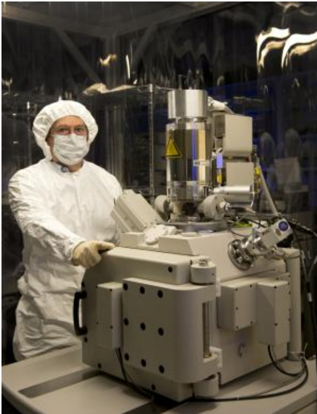
Dr. András Vladár operates the NIST dimensional metrology reference SEM.
