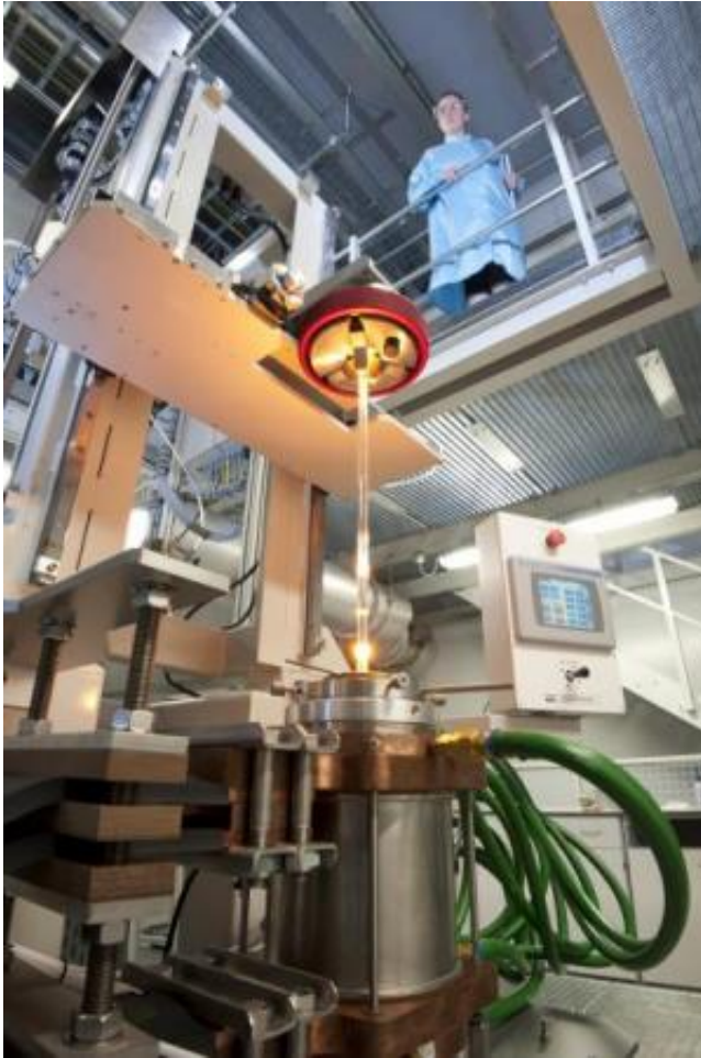
This is a fibre drawing tower at ORC. Credit: University of Southampton
