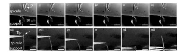
The fracture properties of natural (i-vi) and synthetic spicules (vii-xii) were probed with a micromanipulator, recorded with a scanning electron microscope. The synthetic spicule did not fracture even under extreme loading and deformation conditions.
