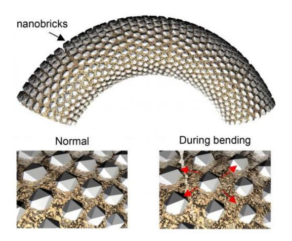
The nanometer size of the calcite bricks facilitates bending of the synthetic spicules. The radius of curvature upon bending is very large compared to the size
