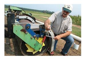
Agricultural engineer Ted Kornecki adjusts the crimping force of his patented smooth roller with oscillating crimping bar. Credit: Ted Kornecki
