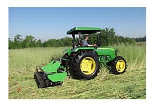
In an experiment at Randle Farms near Auburn, Alabama, technician Corey Kichler operates a two-stage roller/crimper that has a primary drum and a spring-loaded secondary drum with attached equally spaced crimping bars. Credit: Ted Kornecki
