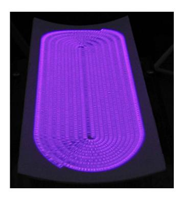
A new 'diffuse coplanar surface barrier discharge' (DCSBD) plasma source (pictured) that rapidly cleans flat polymer sheets in open-air conditions holds great promise for roll-to-roll manufacturing. Credit: 2013 Mirko Černak, Comenius University
