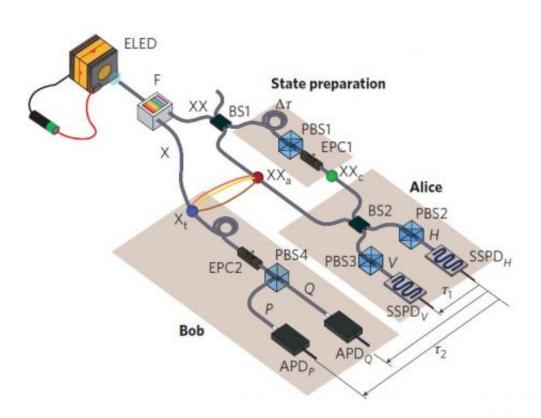
Experimental set-up of the quantum teleportation device including an entangled light-emitting diode (ELED) and an assortment of beam splitters polarization controllers, detectors, and photodiodes. The researchers demonstrated that the device can generate single pairs of entangled photons with advantages compared with using a laser due to the electrical control provided by the ELED. Credit: J. Nilsson, et al. ©2013 Macmillan Publishers Limited. All rights reserved.
