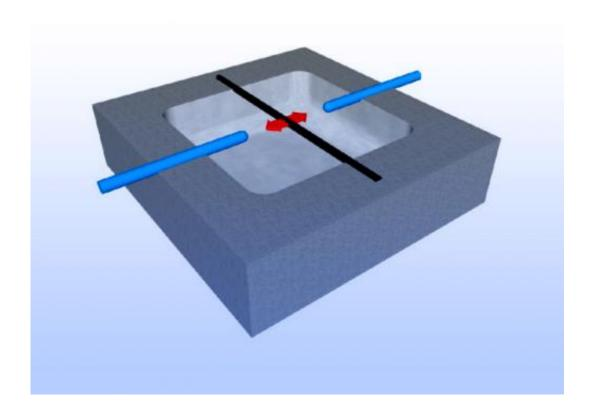
A nanotube (black) can be clamped and excited to vibrate like a guitar string. An electric field (electrodes: blue) ensures that two of the many possible states can be selectively addressed. Credit: Michael J. Hartmann, TUM
