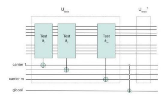
Structure of the Quantum Primality Oracle based on the Miller-Rabin primality test. A series of unitary modules implement a quantum version of the modular exponentiation tests required by the classical test. The total number of tests m is smaller than  $n^2$ . Credit: arXiv:1302.6245 [quant-ph]
