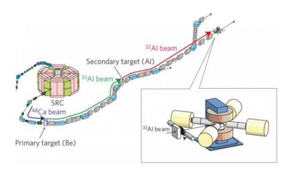
The RIBF facility. Spin-aligned beams of aluminum-32 (32Al) are produced in two stages by first bombarding a beryllium (Be) target with a calcium-48 (48Ca) beam generated by the superconducting ring cyclotron (SRC) to produce an aluminum-33 (33Al) beam, and then bombarding a secondary aluminum target and selecting a narrow band of momentum to produce a 32Al beam with high degree of spin alignment. Credit: 2012 Y. Ichikawa et al.
