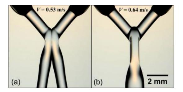
This figure shows two fluid jets merging into one on the right when just a 20 percent speed increase is applied. Credit: Virginia Tech
