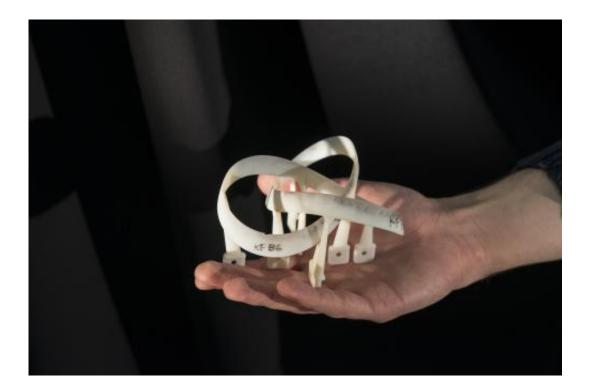
When accelerated to more than 100 g in a specially prepared water tank, hydrofoils like these can generate knotted vortex loops. Physicists have unsuccessfully attempted to create knotted vortices in the laboratory for more than a century. Credit: Robert Kozloff/University of Chicago
