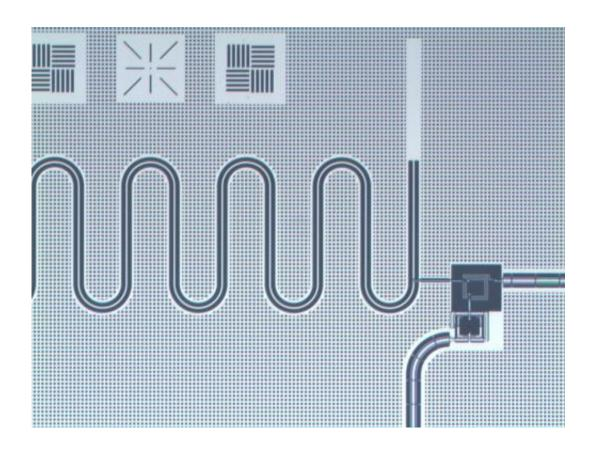
This is a schematic diagram of part of the superconducting chip. The wavy line is the superconducting cavity. The piece in the bottom right is the superconducting switch. Credit: UCSB
