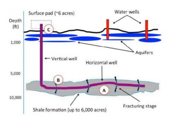
The process of hydraulic fracturing involves drilling a vertical and horizontal well, which can allow the exploration of wide shale formations (up to 6,000 acres) with only a small surface pad (6 acres). Points A, B, C identify the locations for future research opportunities. Credit: Arun Yethiraj and Alberto Striolo, et al. ©2013 American Chemical Society
