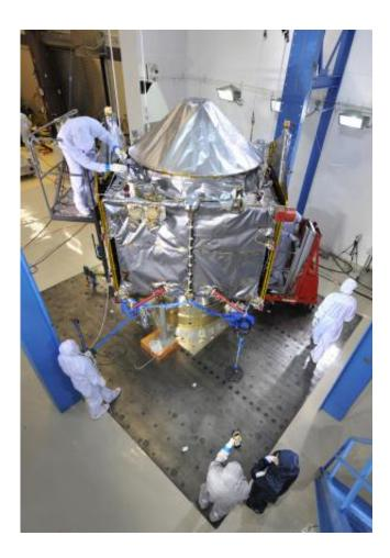
NASA's MAVEN spacecraft undergoes acoustics testing on Feb. 13, 2013 at Lockheed Martin Space Systems' Reverberant Acoustic Laboratory. The environmental test simulates the maximum sound and vibration levels the spacecraft will experience during launch. MAVEN is the next mission to Mars and will be the first mission devoted to understanding the Martian upper atmosphere. Credit: Lockheed Martin
