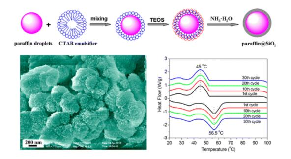
They describe a new approach to using <u>paraffin</u> as a PCM. Made from petroleum, paraffin is a waxy material that absorbs heat, melts into a liquid and releases heat as it solidifies. It involves encapsulating paraffin into tiny spheres of silicon dioxide, the stuff of beach sand. The microencapsulated paraffin has several advantages, including a large
