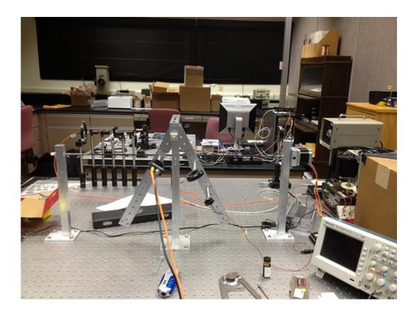
The right leg of this optical-sensing device contains a light source that shines a beam up into a prism. The sample rests on the top of the prism. Eventually, the beam is sent down the other leg of the device into a photon detector, which helps analyze the sample.
