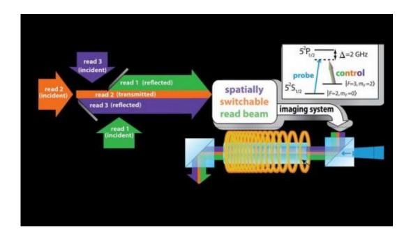
Experimental setup for multiple-readout gradient echo memory (GEM) experiment. The three read beams are combined using edge-coated mirrors and imaged into the memory cell. The probe and control beams are combined using a polarizing beam splitter (PBS). Inset: The rubidium energy levels involved in the absorption of the control and probe (image) beams.
