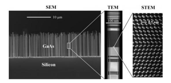
Nanowire crystals are used as the solar cells. The image (left) shows a SEM (Scaning Electron Microscope) image of GaAs nanowire crystal grown on a Silicon substrate. A TEM (Transmission Electron Microscope) image (middle) shows a single nanowire. Further zooming in on the crystal structure, using STEM (Scanning Transmission Electron Microscope) imaging, shows the actual atomic columns (right). Credit: Niels Bohr Institute
