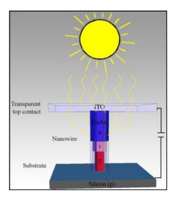
The figure shows that the sun's rays are drawn into a nanowire, which stands on a substrate. At a given wavelength the sunlight is concentrated up to 15 times. Consequently, there is great potential in using nanowires in the development of future solar cells. Credit: Niels Bohr Institute
