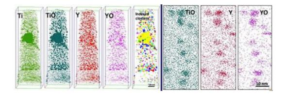
EMSL's LEAP® 4000 atom probe tomography instrument provides a 3-D view of atomic-level physical and chemical interactions in metallic elements, such as the irradiated ODS steels used in this study. The APT work revealed clear images of the nanoclusters for better comparisons. Here, the 14YWT, 100 dpa sample (left) was ion irradiated (450°C), while the 9CrODS sample (right) was neutron irradiated at 500°C.
