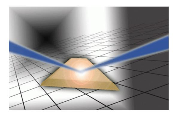
An ultraviolet light pulse hits the titanium dioxide crystal. The laser pulse induces a redistribution of weakly bound electrons, which leads to a shift of the equilibrium position of the atoms in the crystal lattice. Credit: Thorsten Naeser
