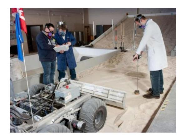
Undated image provided by NASA on March 26, 2013 shows NASA's Colin Creager testing soil with a cone penetrometer at Glenn Research Center's Simulated Lunar Operations facility in Ohio. A self-sustaining mechanised colony that mines and exports resources from the Moon could be a reality within a generation, helping to meet demand for materials key to innovation on Earth.
