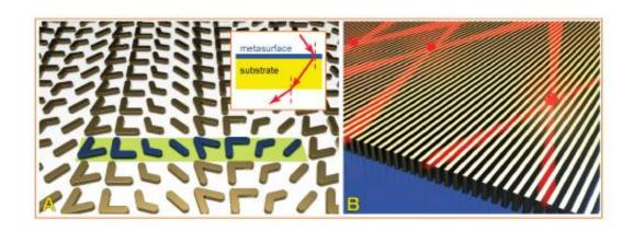
This schematic view of a nanoantenna array (A), at left, is an example of new plasmonic metasurfaces that are promising for various advances, including a possible "hyperlens" that could make optical microscopes 10 times more powerful. At right (B) is a "hyperbolic metasurface," a tiny metallic grating for enhancing "quantum emitters," which could make possible future quantum information systems far more powerful than today's computers. Credit: Birck Nanotechnology Center, Purdue University
