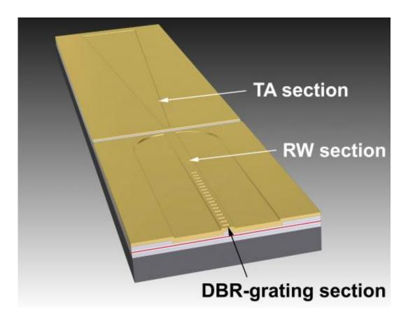
Within the ridge waveguide (RW section) high-quality radiation is generated, which is amplified within the tapered section (TA section) – this tapered laser thus combines excellent beam quality with very high output power. Credit: FBH/D. Feise
