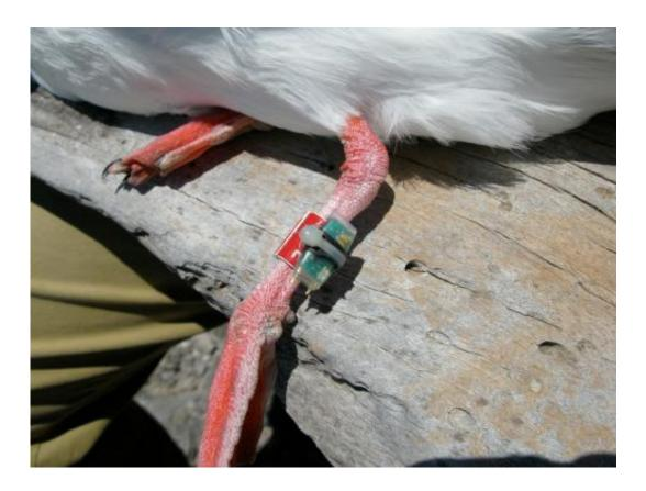
Microsensors are attached to the gulls' legs, transmitting data to the researchers on the birds' swimming phases. Credit: MPI for Ornithology
