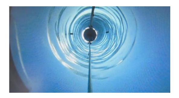
A video camera on a NASA-designed-and-funded mini-submarine captured this view as it descended a 2,600-foot-deep (800-meter-deep) borehole to explore Antarctica's subglacial Lake Whillans. The international Whillans Ice Stream Subglacial Access Research Drilling (WISSARD) project was designed to gain insights into subglacial biology, climate history and modern ice sheet behavior. Credit: NASA/JPL-Caltech
