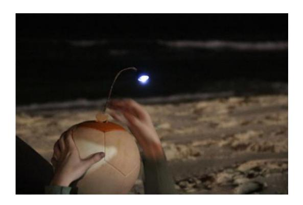
(Phys.org) —A collaboration between groups Uncharted Play and Power the World, has resulted in the creation of a soccer ball generator they call the SOCCKET—when used, it generates enough electricity to power an attachable LED lamp for up to three hours. The team has been testing their ball for over a year in impoverished regions of North and South
