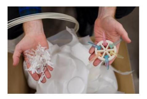
To make the lab equipment on the right, Michigan Tech's Joshua Pearce first shredded milk jugs and then turned them into plastic filament. A 3D printer transformed the filament into a DremelFuge, a centrifuge for rotary tools. Credit: Sarah Bird/Michigan Technological University
