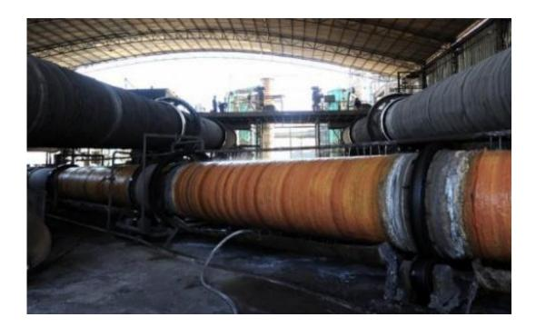
Rare earths undergoing processing in large steel pipes are cooled off with dripping water at a privately-owned factory on the outskirts of Baotou city in Inner Mongolia, northwest China on April 21, 2011.
